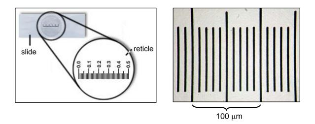
**Figure 6** - Nikon microscope slide scale (left) and the corresponding microscopic digital image (right). The larger vertical bars define distance intervals of 100  $\mu$ m.
