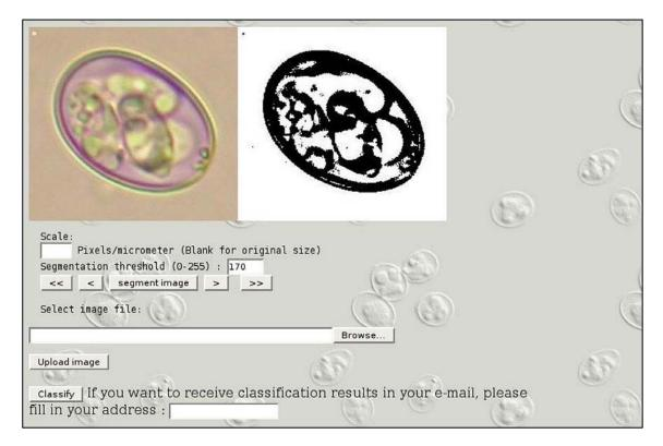
**Figure 4** – Too high segmentation values result in no visible line of contour. In fact, the delimited area can be seen as a small circle on the upper left corner of the picture on the left.
