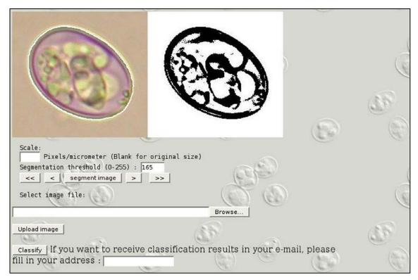
**Figure 2** – An adequate segmentation value yields a well defined white contour line surrounding the oocyst image (picture on the left).
