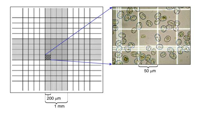
**Figure 7** - The Neubauer counting chamber (hemocytometer) reticle (left) and the corresponding microscopic digital image (right). The small squares of the reticle present a side length of 50  $\mu$ m. Oocysts of *E. acervulina* (larger diameter of 19±1.3  $\mu$ m) are displayed for size comparison purpose only.
